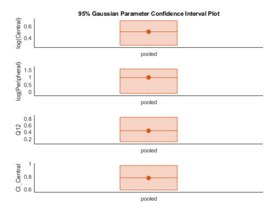
Plot all the confidence interval results together. By default, the confidence interval for each parameter estimate is plotted in a separate axes. Vertical dotted lines group confidence intervals of parameter estimates that were computed in a common fit. Parameter bounds defined in the original fit are marked by square brackets (if visible in the parameter range being plotted).
