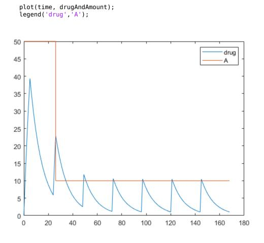
Alternatively, you can allow the ongoing dose event to finish before applying the new dose amount by setting EventMode to 'continue'.
