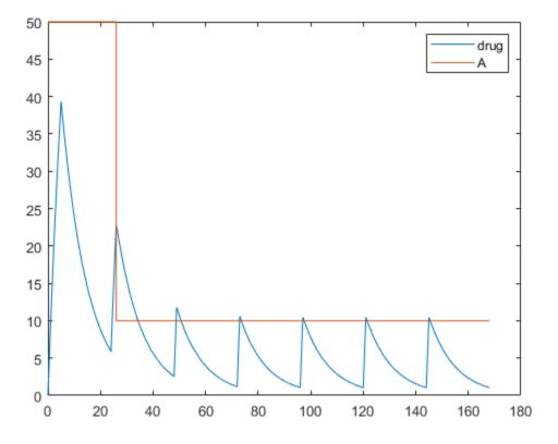
Alternatively, you can allow the ongoing dose event to finish before applying the new dose amount by setting EventMode to 'continue'.
