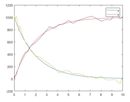
You can also apply a different error model to each state, which is a column in sd. Suppose you want to apply the custom error model (em) to the first column (species x data) and the proportional error model to the second column (species z data).
